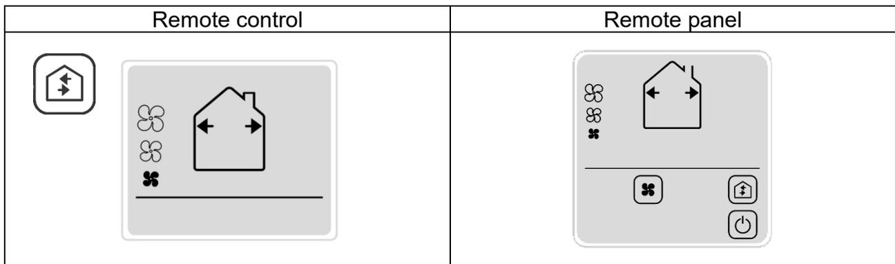
By pressing the specific function button all the units will constantly run in extraction with the possibility to change the speed as required.
