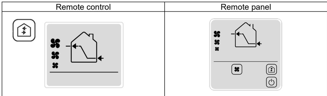
In this mode the units generate a continuous air flow going from SLAVE OPPOSITE TO MASTER to MASTER or SLAVE SAME AS MASTER units excluding heat recovery.
