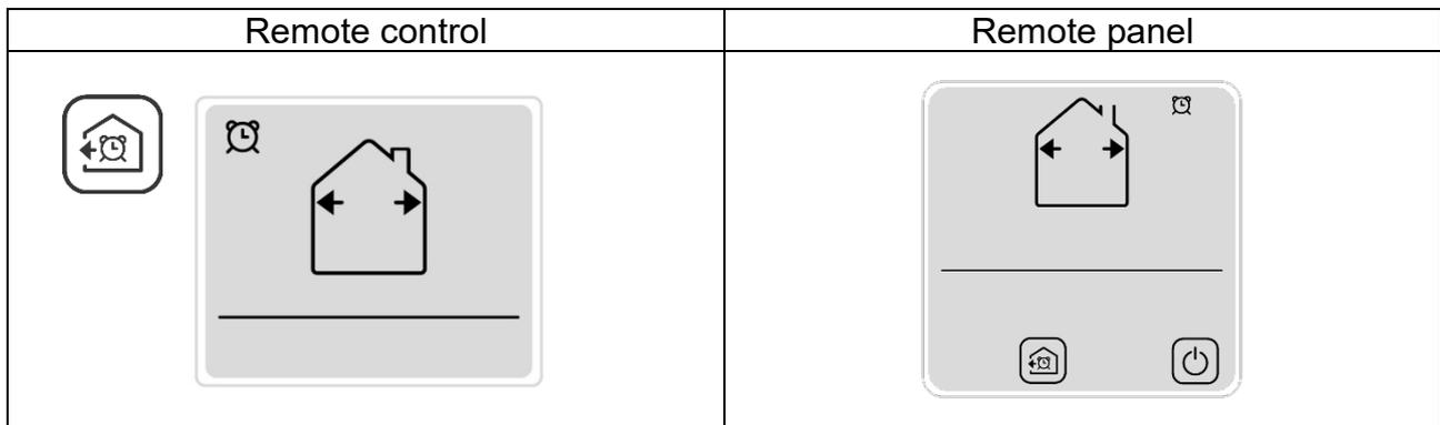
By pressing this button in any of the modes all the products will run in extraction at the maximum speed for 20 minutes, at the end of the cycle they will resume the previous set mode.
