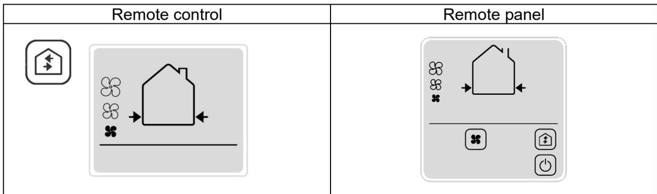
By pressing the specific function button all the units will constantly run in intake with the possibility to change the speed as required.
