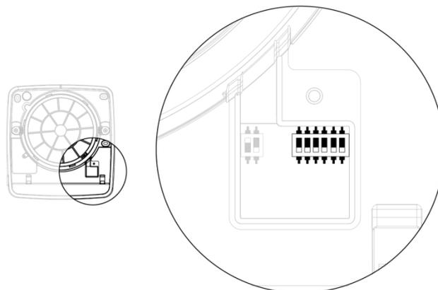
**WARNING:** factory setting of dip switches is 0 (OFF), thus recommended to set on 1 (ON) at least one of the dip switches to uniquely codify the system.
