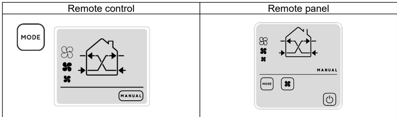
In this mode the sensors are disabled and the units will run with heat recovery. The end user can select the desired speed to run the units and this condition remains until a different command is entered.
