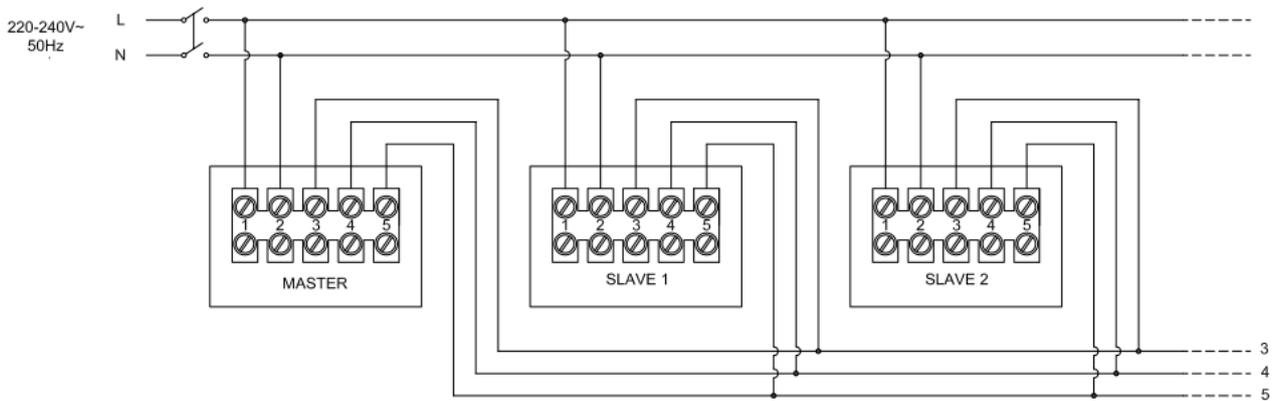
Warning: Humidity and twilight sensors will detect the values from the first unit connected. In case of a system with long wires or with a lot of electric/electronic equipment may cause signal disturbance to use shielded cables and connect a termination resistor of 120ohm on pin 3 and 4 of the terminal block of the last SLAVE.
