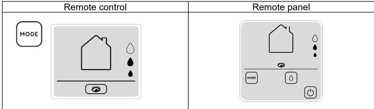
In this mode both humidity and twilight sensors are active, the units will be normally in stand-by with front panel closed, so that when the humidity level in the room exceeds the set threshold the units start running in extraction.
