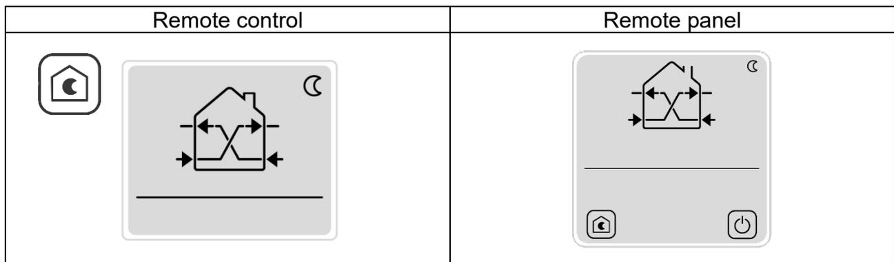
In this mode all the units will run at the night speed with heat recovery until another command is entered.
