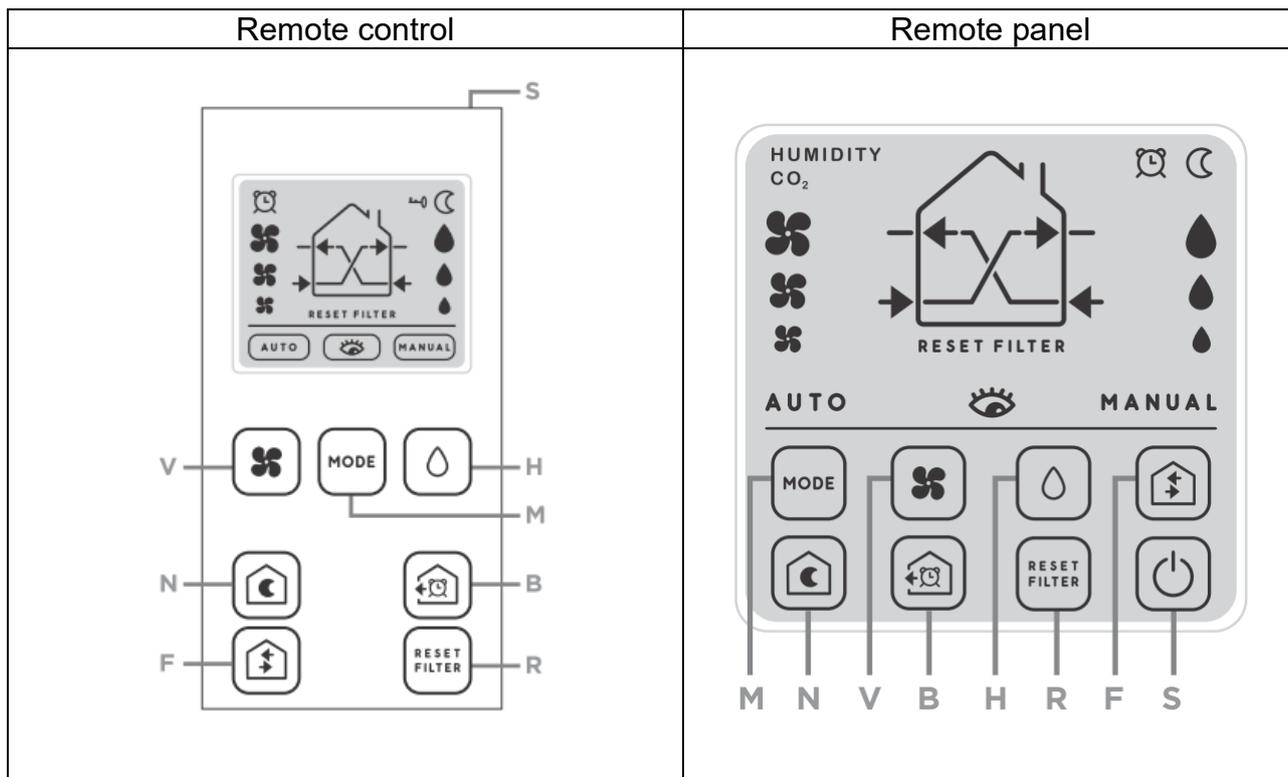
**WARNING (Remote control):** the remote control gets into stand-by mode after being inactive for 60 seconds when the icon with key appears on display. To unlock press the button (S) on the upper side of the remote control.
